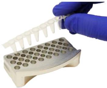
Pull out the collection tube rack and place 0.2 ml PCR tubes firmly into the rack.
