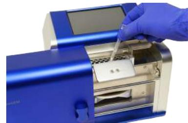
Load the cartridges into the holes of the cartridge tray in the same position where you placed the collection tubes.
