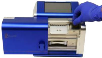
The door of the PDQeX slides horizontally left and right. The door will lock during operation or UV decontamination.
