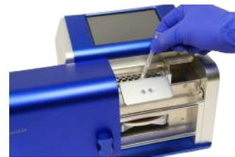
Load the cartridges into the holes of the cartridge tray in the same position where you placed the collection tubes.
