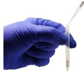
Load your sample into the PDQeX extractor cartridge.
