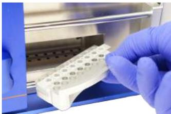
Replace the rack into its slot in the PDQeX and firmly push into place.
