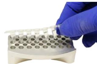
When the program is finished, remove the PDQeX extractor cartridges and dispose. Slide out the drawer.
